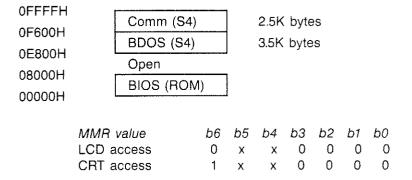
The same situation as in the 32K CP/M kernel mode exists here, and the same methods used there are used in this mode.
