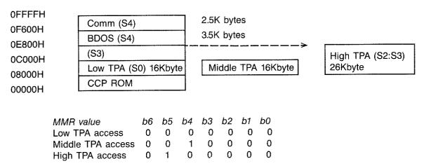
The CCP in the 64K CP/M configuration handles the TPA by swapping one of the low, middle, or high TPA RAM segments into the CPU addressing space at 08000H through 0BFFFH. Since the loading of the application program is made in 128 byte increments, there is no chance that the DMA address would be set across the boundaries of any TPA segment.
