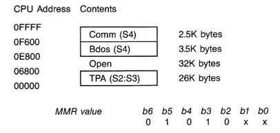
The size of the TPA is 26K bytes, which is the same TPA size of a 31K CP/M when the CCP area is overwritten.
