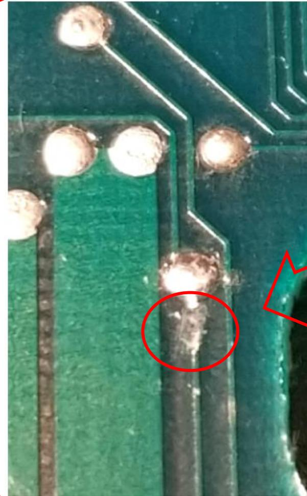
Pin 37 of the CPU drives the system clock signal. That must be disconnected. One way is to cut the clock track at the indicated location. There are other ways too. But this might be the easiest.
