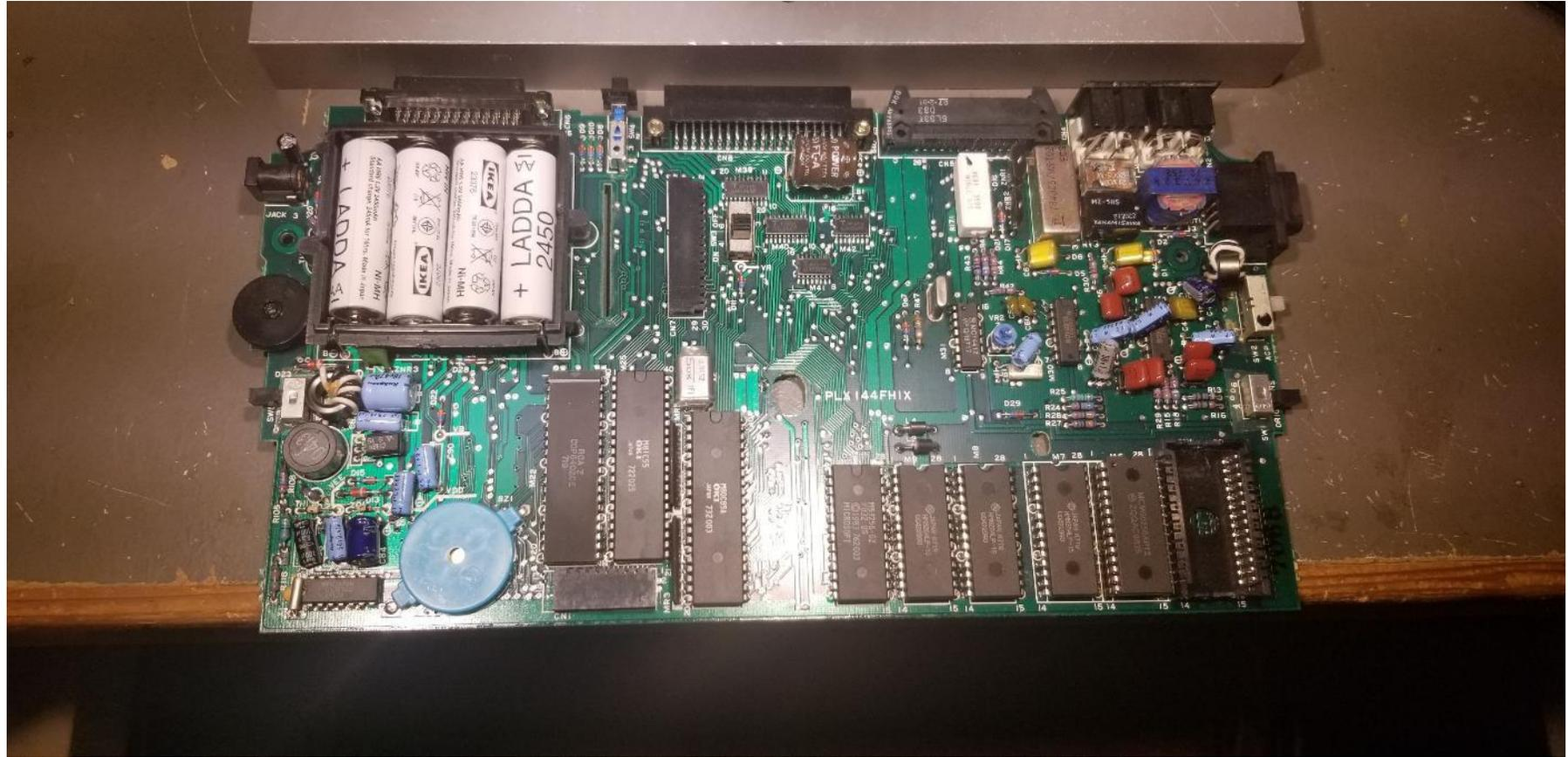
Here we have removed the main PCB from the case. Also, removed the ribbon cables carefully.
