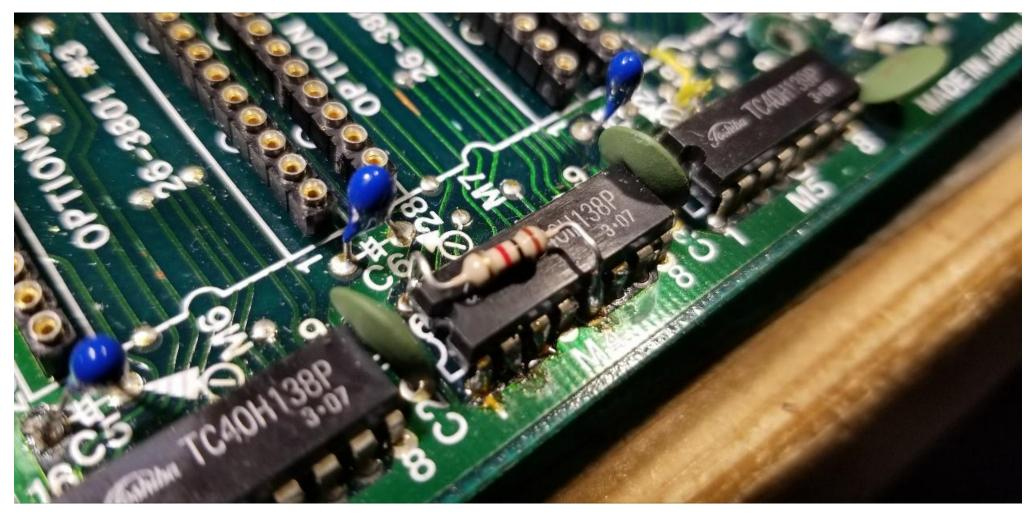
Bend leads and trim to fit 1kohm resistor on top of M7. Connect 1K from pin 16 (+5V) to pin 6 (A\*). This should pull A\* to 3.5V or higher.
