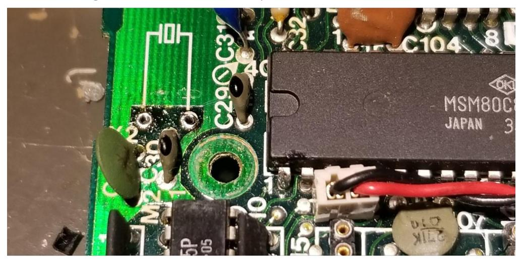
Remove the M100 PCB from the case. Using whatever means, remove the crystal and clean out the vias. Save crystal if you want to revert.
