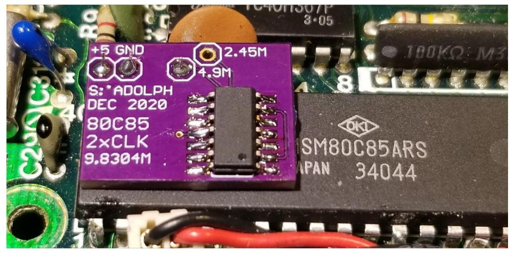
Slide the divider PCB onto the three pins as indicated. Solder lightly as to not dislodge the wires from the CPU.
