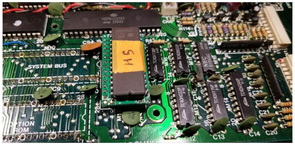
Install new Main ROM using adapter. Use an EPROM that is 150nsec or faster. Image can be stock, or modified to suit. I'm using the hardware scroll patch.
