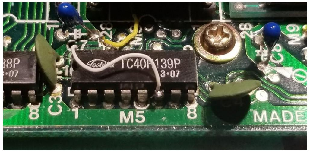
Solder a short wire from pin 16 to pin 6 of M5. This will permanently pull A\* signal to +5V, and consumes about 4mA. This enables slower SRAM to work.
