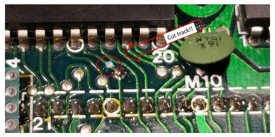
Cut track carefully as indicated, to isolate the clock fed from pin 37 of the CPU. This is easily reversed with a single strap wire if needed.
