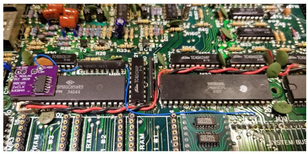
Run a wire from the via right next to the clock track cut, to the 2.45M pin on the clock divider PCB.
