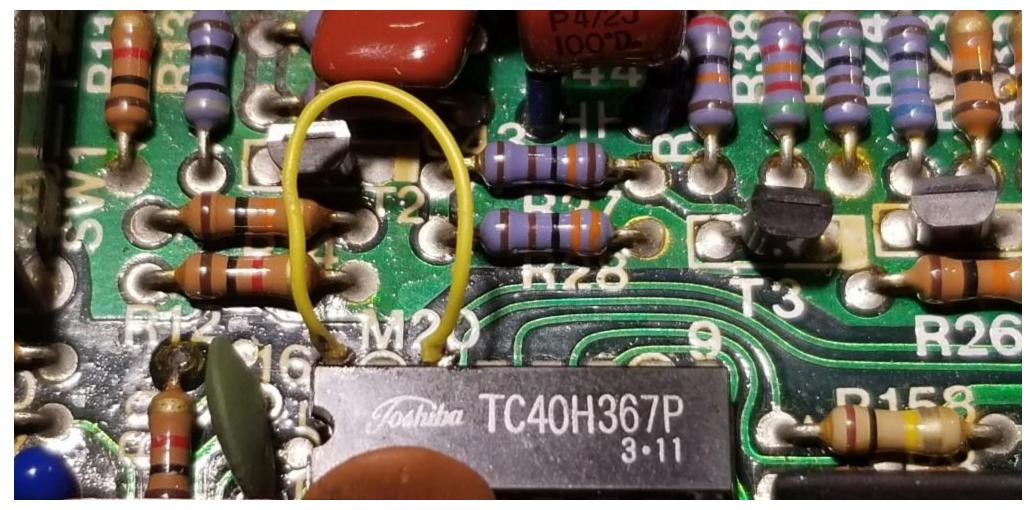
Solder a short wire from pin 16 to pin 4 of M20. This drives A\* high to the chip select circuits, which in turn speeds up the access to the SRAM.
