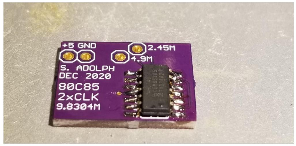
Solder the 74HC74D IC to the divider PCB.
