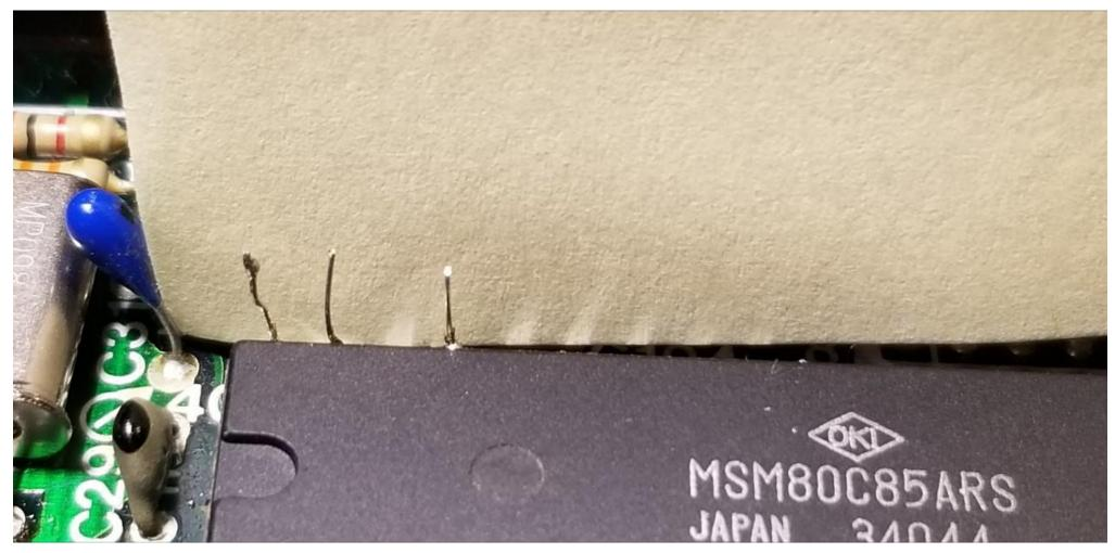
Solder 3 short wires vertically to pins 40, 39 and 37 on the CPU, as shown.
