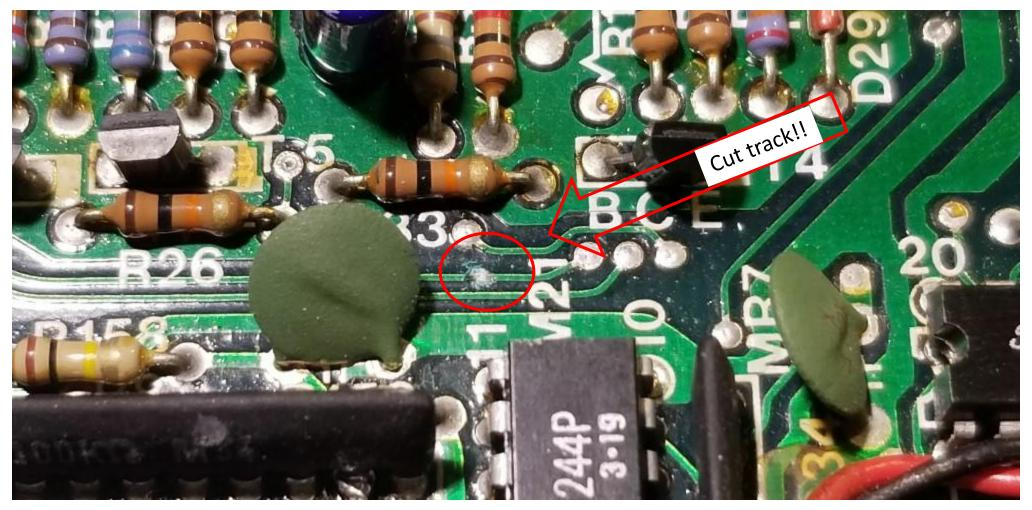
Cut track as indicated. This disconnects the input to the M20 A\* buffer at pin 14.
